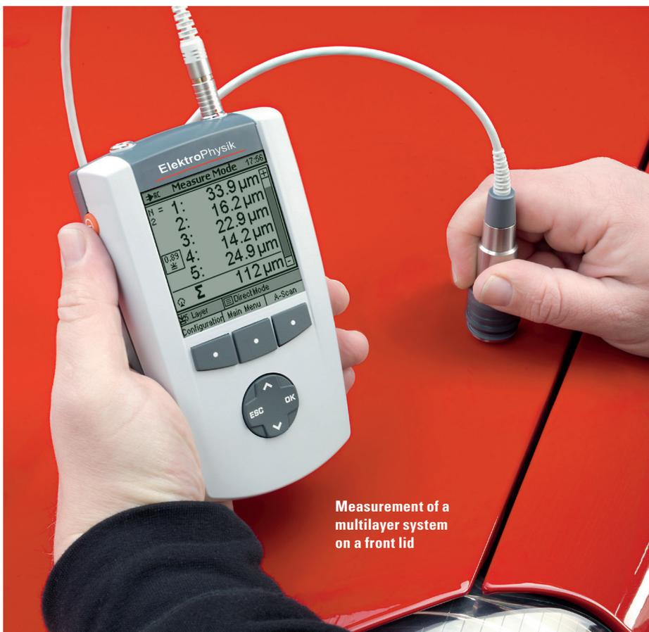
Measurement of a multilayer system on a front lid
