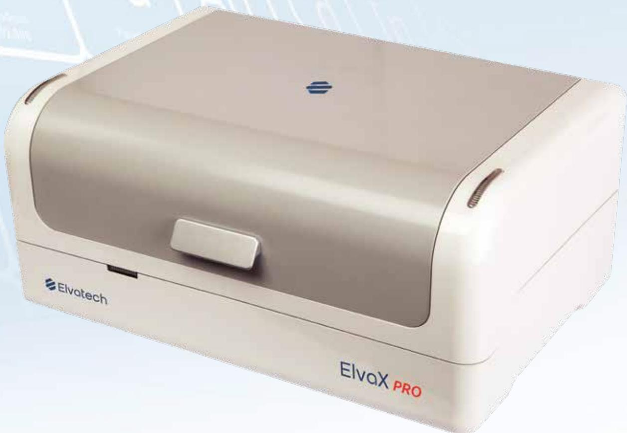
ElvaX Pro is the next-generation benchtop X-ray fluorescence analyzer. It offers a new level of analysis accuracy, speed and detection limits for a wide range of elements from Na(11) to U(92) due to the new 60kV, 1000 uAmp X-ray tube and the ultra large area Fast SDD detector. Powerful hardware combined with unique software algorithms make ElvaX Pro a multipurpose lab instrument for elemental analysis of various materials including solids, powders, liquids etc.
