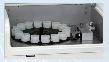
The optional automatic 16-positions sample changer coupled with the fast measurement increases the productivity of your lab up to 1000 samples per workday.
