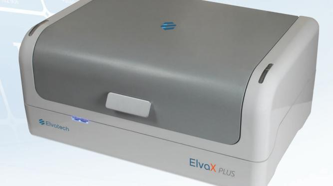
ElvaX Plus spectrometer is a desktop energy-dispersive X-ray fluorescence (EDXRF) analyzer with extended element range from Na (Z=11) to U (Z=92). The Helium purge system and the automatic primary filter changer combined with the large area SDD detector are used to allow effective registration of the light elements spectra.
