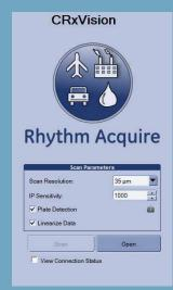
3 Insert the imaging plate(s) to start the cycle
